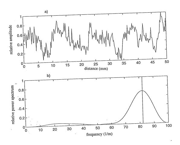
Figure C.14. (a) The spatially, amplitude modulated, received signal plotted against position along a glass plate's surface (250 RMS data points, 50 mm scan distance). (b) The power spectrum of the signal from (a) plotted against the spatial frequency (1/distance). The vertical line indicates the theoretically estimated spatial beat frequency,  $82.2 \, m^{-1}$ . The frequency used was  $0.80 \, MHz$ . The experimentally measured spatial beat frequency is  $81.8 \, m^{-1}$ .
