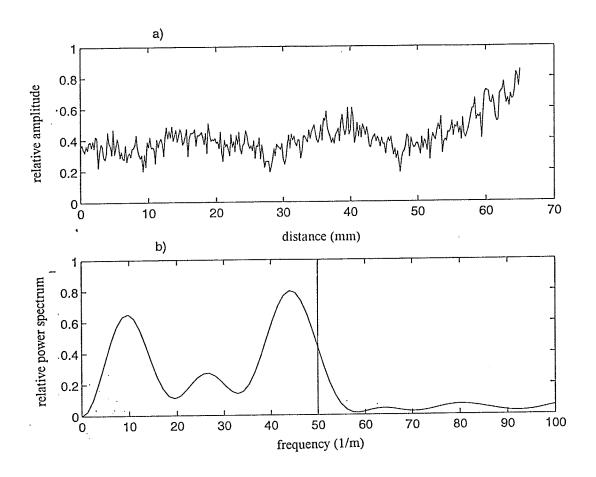
Figure C.10. (a) The spatially, amplitude modulated, received signal plotted against position along a brass plate's surface (350 RMS data points, 70 mm scan distance). (b) The power spectrum of the signal from (a) plotted against the spatial frequency (1/distance). The vertical line indicates the theoretically estimated spatial beat frequency,  $50.0 \, m^{-1}$ . The frequency used was  $1.00 \, MHz$ . The experimentally measured spatial beat frequency is  $45.2 \, m^{-1}$ .
