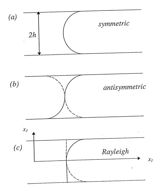
Figure 2. A sketch of the  $x_1$  particle displacements corresponding to the neighbourhood of the intersections of the long dashed horizontal lines in Fig. 1 with the dispersion curves. The solid lines indicate that the modes are in phase, while the dashed lines indicate that they are  $\pi$  out of phase. (a) symmetric mode; (b) antisymmetric mode; (c) algebraic sum of the two modes.
