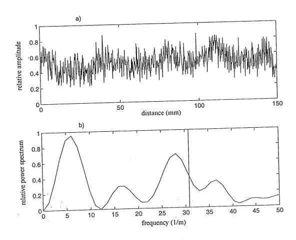
Figure C.11. (a) The spatially, amplitude modulated, received signal plotted against position along a brass plate's surface (750 RMS data points, 150 mm scan distance). (b) The power spectrum of the signal from (a) plotted against the spatial frequency (1/distance). The vertical line indicates the theoretically estimated spatial beat frequency,  $30.8 \ m^{-1}$ . The frequency used was  $1.20 \ MHz$ . The experimentally measured spatial beat frequency is  $28.1 \ m^{-1}$ .
