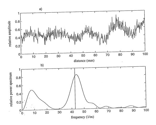
Figure C.16. (a) The spatially, amplitude modulated, received signal plotted against position along a glass plate's surface (500 RMS data points, 100 mm scan distance). (b) The power spectrum of the signal from (a) plotted against the spatial frequency (1/distance). The vertical line indicates the theoretically estimated spatial beat frequency,  $42.9 \ m^{-1}$ . The frequency used was  $1.00 \ MHz$ . The experimentally measured spatial beat frequency is  $44.0 \ m^{-1}$ .
