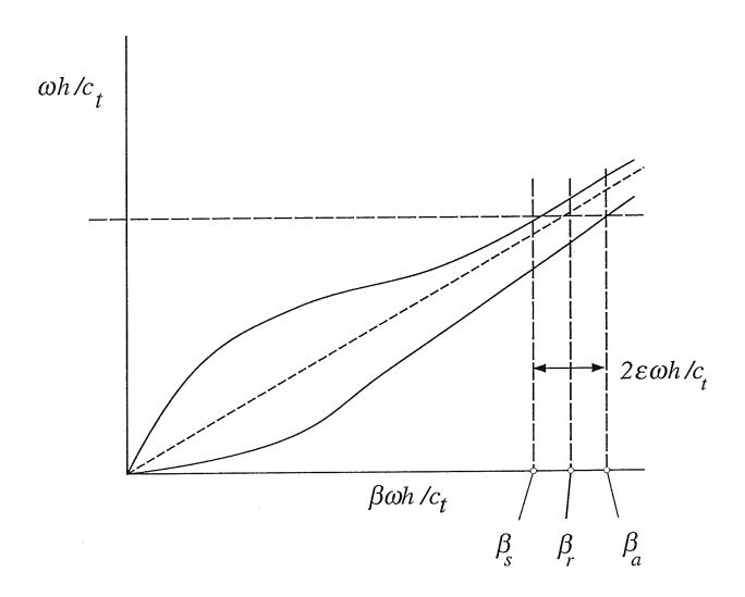
Figure 1. The dispersion relation for the two lowest modes of an elastic plate. The upper curve is the symmetric mode and the lower curve is the anti-symmetric mode. The beatlength  $L = \pi c_t / (\varepsilon \omega)$ . Figure 2 indicates the particle displacement in the neighbourhood of the intersections of the long dashed horizontal line with the dispersion curves.
