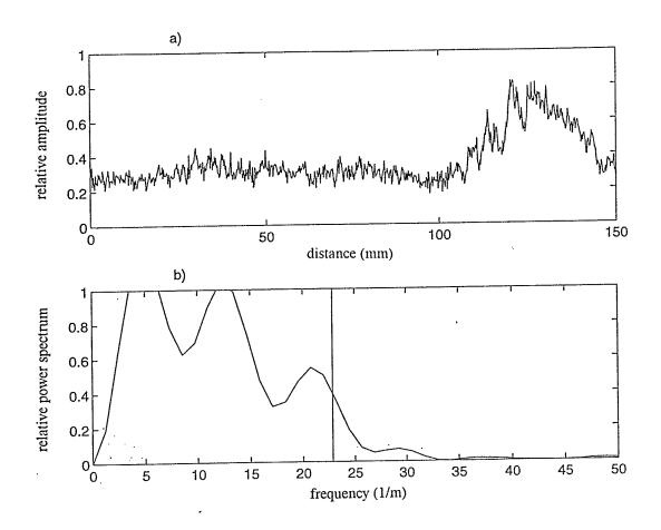
Figure C.12. (a) The spatially, amplitude modulated, received signal plotted against position along a brass plate's surface (750 RMS data points, 150 mm scan distance). (b) The power spectrum of the signal from (a) plotted against the spatial frequency (1/distance). The vertical line indicates the theoretically estimated spatial beat frequency,  $22.9 \ m^{-1}$ . The frequency used was 1.33 MHz. The experimentally measured spatial beat frequency is  $22 \ m^{-1}$ .
