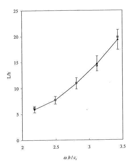
Figure 17. A plot of L/h against  $\omega h/c_t$  for glass. The data points, represented by squares, are the measured results. The data points represented by diamonds are the theoretically predicted results. A  $\pm$  10% error bar is attached to each of the theoretically predicted results.
