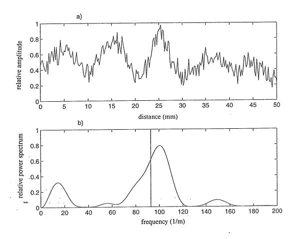
Figure C.1. (a) The spatially, amplitude modulated, received signal plotted against position along an aluminum plate's surface (250 RMS data points, 50 mm scan distance). (b) The power spectrum of the signal from (a) plotted against the spatial frequency (1/distance). The vertical line indicates the theoretically estimated spatial beat frequency, 92.9  $m^{-1}$ . The frequency used was 1.2 MHz. The experimentally measured spatial beat frequency is  $101.3 m^{-1}$ .
