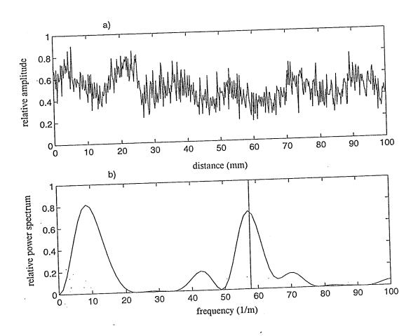
Figure C.15. (a) The spatially, amplitude modulated, received signal plotted against position along a glass plate's surface (500 RMS data points, 100 mm scan distance). (b) The power spectrum of the signal from (a) plotted against the spatial frequency (1/distance). The vertical line indicates the theoretically estimated spatial beat frequency, 57.9  $m^{-1}$ . The frequency used was 0.90 MHz. The experimentally measured spatial beat frequency is 57.4  $m^{-1}$ .
