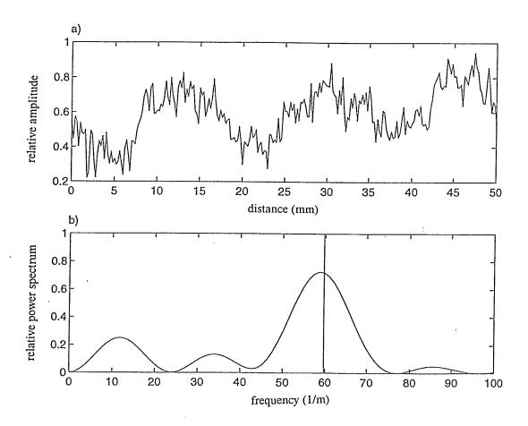
Figure 13. Representative data for brass, case 4 of Table 2. (a) The spatially, amplitude modulated, received signal plotted against position along the plate's surface (250 RMS data points, 50 mm scan distance). (b) The power spectrum of the signal from (a) plotted against the spatial frequency (1/distance). The vertical line indicates the theoretically estimated spatial beat frequency,  $L = \pi c_t / (\varepsilon \omega)$ .
