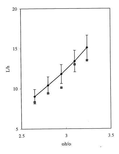
Figure 15. A plot of L/h against  $\omega \, h/c_t$  for aluminum. The data points, represented by squares, are the measured results. The data points represented by diamonds are the theoretically predicted results. A  $\pm$  10% error bar is attached to each of the theoretically predicted results.
