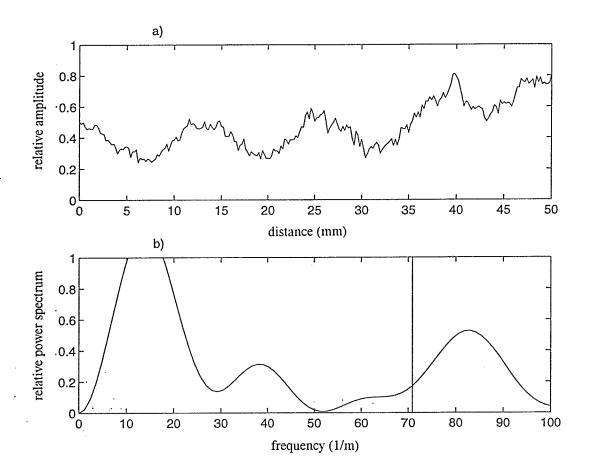
Figure C.3. (a) The spatially, amplitude modulated, received signal plotted against position along an aluminum plate's surface (250 RMS data points, 50 mm scan distance). (b) The power spectrum of the signal from (a) plotted against the spatial frequency (1/distance). The vertical line indicates the theoretically estimated spatial beat frequency,  $70.9 \, m^{-1}$ . The frequency used was 1.33 MHz. The experimentally measured spatial beat frequency is  $83.0 \, m^{-1}$ .
