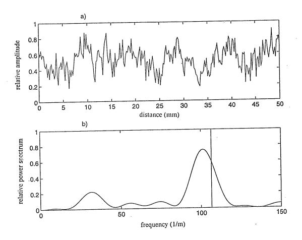
Figure C.13. (a) The spatially, amplitude modulated, received signal plotted against position along a glass plate's surface (250 RMS data points, 50 mm scan distance). (b) The power spectrum of the signal from (a) plotted against the spatial frequency (1/distance). The vertical line indicates the theoretically estimated spatial beat frequency,  $106.5 \, m^{-1}$ . The frequency used was  $0.70 \, MHz$ . The experimentally measured spatial beat frequency is  $101.3 \, m^{-1}$ .
