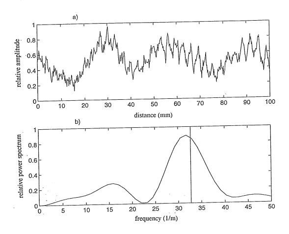
Figure C.17. (a) The spatially, amplitude modulated, received signal plotted against position along a glass plate's surface (500 RMS data points, 100 mm scan distance). (b) The power spectrum of the signal from (a) plotted against the spatial frequency (1/distance). The vertical line indicates the theoretically estimated spatial beat frequency,  $32.7 m^{-1}$ . The frequency used was 1.10 MHz. The experimentally measured spatial beat frequency is  $31.7 m^{-1}$ .
