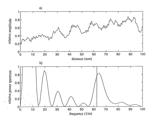
Figure C.4. (a) The spatially, amplitude modulated, received signal plotted against position along an aluminum plate's surface (500 RMS data points, 100 mm scan distance). (b) The power spectrum of the signal from (a) plotted against the spatial frequency (1/distance). The vertical line indicates the theoretically estimated spatial beat frequency, 62.5  $m^{-1}$ . The frequency used was 1.4 MHz. The experimentally measured spatial beat frequency is 64.7  $m^{-1}$ .
