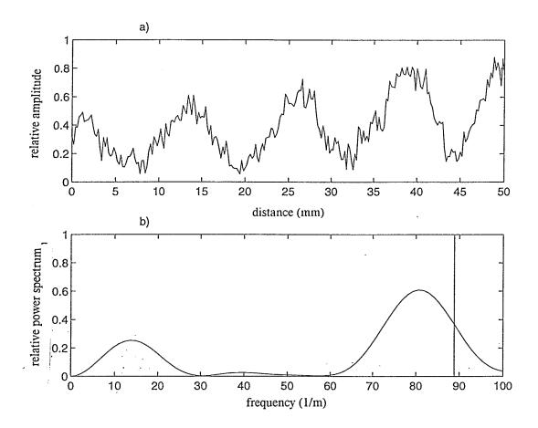
Figure C.7. (a) The spatially, amplitude modulated, received signal plotted against position along a brass plate's surface (250 RMS data points, 50 mm scan distance). (b) The power spectrum of the signal from (a) plotted against the spatial frequency (1/distance). The vertical line indicates the theoretically estimated spatial beat frequency,  $88.9 \, m^{-1}$ . The frequency used was  $0.80 \, MHz$ . The experimentally measured spatial beat frequency is  $80.6 \, m^{-1}$ .
