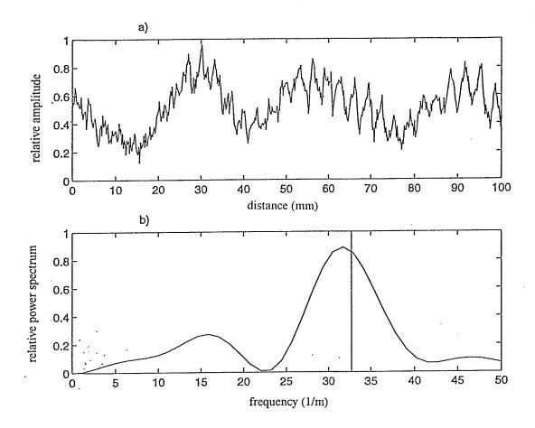
Figure 14. Representative data for glass, case 5 of Table 3. (a) The spatially, amplitude modulated, received signal plotted against position along the plate's surface (500 RMS data points, 100 mm scan distance). (b) The power spectrum of the signal from (a) plotted against the spatial frequency (1/distance). The vertical line indicates the theoretically estimated spatial beat frequency,  $L = \pi c_t / (\varepsilon \omega)$ .
