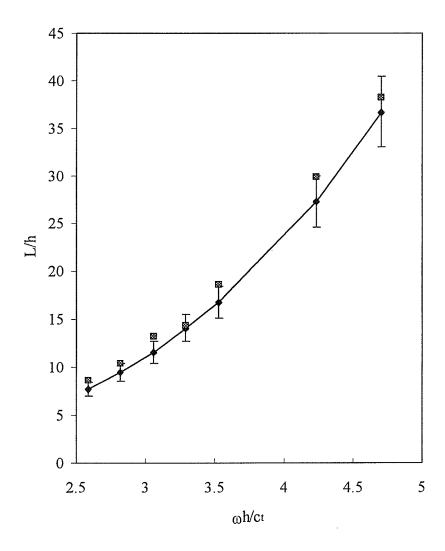
Figure 16. A plot of L/h against  $\omega h/c_t$  for brass. The data points, represented by squares, are the measured results. The data points represented by diamonds are the theoretically predicted results. A  $\pm$  10% error bar is attached to each of the theoretically predicted results.
