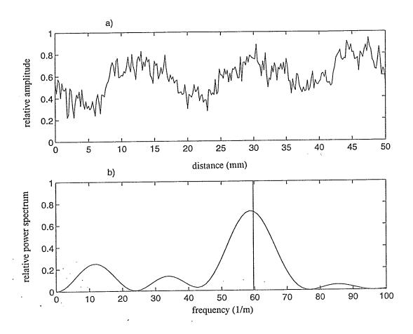
Figure C.9. (a) The spatially, amplitude modulated, received signal plotted against position along a brass plate's surface (250 RMS data points, 50 mm scan distance). (b) The power spectrum of the signal from (a) plotted against the spatial frequency (1/distance). The vertical line indicates the theoretically estimated spatial beat frequency,  $59.7 \, m^{-1}$ . The frequency used was  $0.93 \, MHz$ . The experimentally measured spatial beat frequency is  $58.6 \, m^{-1}$ .
