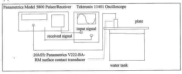
Figure 3. Schematic diagrams of the experimental setup for measuring (a) the longitudinal speed and (b) shear speed in an elastic plate.
