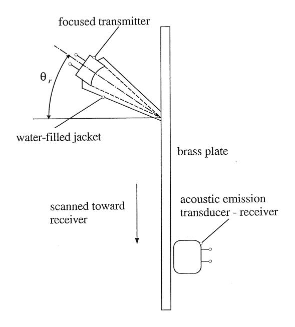
Figure 5. A sketch of the experimental arrangement viewed from the top. The central axis of the focused transducer makes an angle  $\theta_r$  with the vertical. The sound is coupled to the plate by means of a water-filled jacket. The plate is otherwise loaded only by the surrounding air. The focal point is placed at the plate surface and moved toward the stationary receiving transducer.
