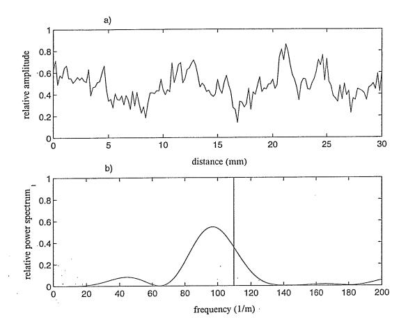
Figure C.6. (a) The spatially, amplitude modulated, received signal plotted against position along a brass plate's surface (150 RMS data points, 30 mm scan distance). (b) The power spectrum of the signal from (a) plotted against the spatial frequency (1/distance). The vertical line indicates the theoretically estimated spatial beat frequency,  $109.8 \, m^{-1}$ . The frequency used was  $0.73 \, MHz$ . The experimentally measured spatial beat frequency is  $97.7 \, m^{-1}$ .
