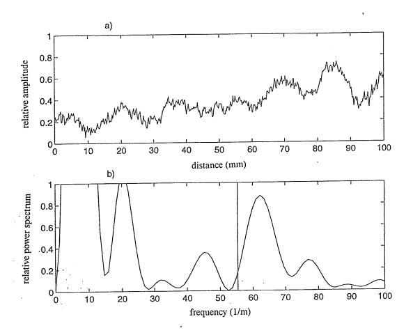
Figure C.5. (a) The spatially, amplitude modulated, received signal plotted against position along an aluminum plate's surface (500 RMS data points, 100 mm scan distance). (b) The power spectrum of the signal from (a) plotted against the spatial frequency (1/distance). The vertical line indicates the theoretically estimated spatial beat frequency,  $55.4 \, m^{-1}$ . The frequency used was  $1.46 \, MHz$ . The experimentally measured spatial beat frequency is  $62.3 \, m^{-1}$ .
