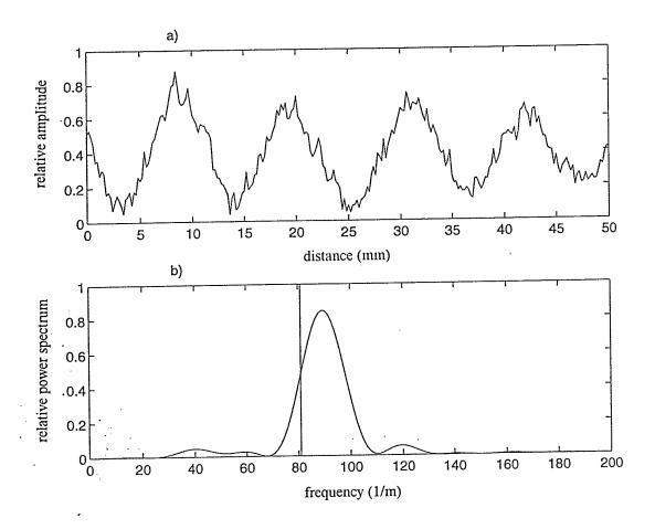
Figure C.2. (a) The spatially, amplitude modulated, received signal plotted against position along an aluminum plate's surface (250 RMS data points, 50 mm scan distance). (b) The power spectrum of the signal from (a) plotted against the spatial frequency (1/distance). The vertical line indicates the theoretically estimated spatial beat frequency,  $80.9 \, m^{-1}$ . The frequency used was  $1.26 \, MHz$ . The experimentally measured spatial beat frequency is  $89.1 \, m^{-1}$ .
