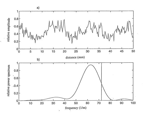
Figure C.8. (a) The spatially, amplitude modulated, received signal plotted against position along a brass plate's surface (250 RMS data points, 50 mm scan distance). (b) The power spectrum of the signal from (a) plotted against the spatial frequency (1/distance). The vertical line indicates the theoretically estimated spatial beat frequency,  $72.3 \, m^{-1}$ . The frequency used was  $0.86 \, MHz$ . The experimentally measured spatial beat frequency is  $63.5 \, m^{-1}$ .
