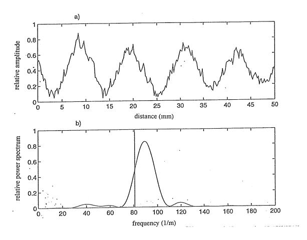
Figure 12. Representative data for aluminum, case 2 of Table 1. (a) The spatially, amplitude modulated, received signal plotted against position along the plate's surface (250 RMS data points, 50 mm scan distance). (b) The power spectrum of the signal from (a) plotted against the spatial frequency (1/distance). The vertical line indicates the theoretically estimated spatial beat frequency,  $L = \pi c_t / (\varepsilon \omega)$ .
