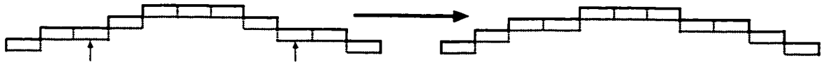
Figure 7.24: Illustration of the additional filter applied to the complex ocean surface curve.
