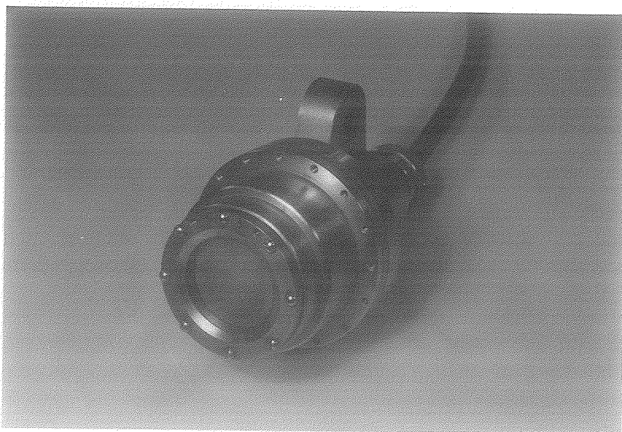
Fig. 18. Transducer No. 2: Large Aperture, Plane Wave Acoustic Source
